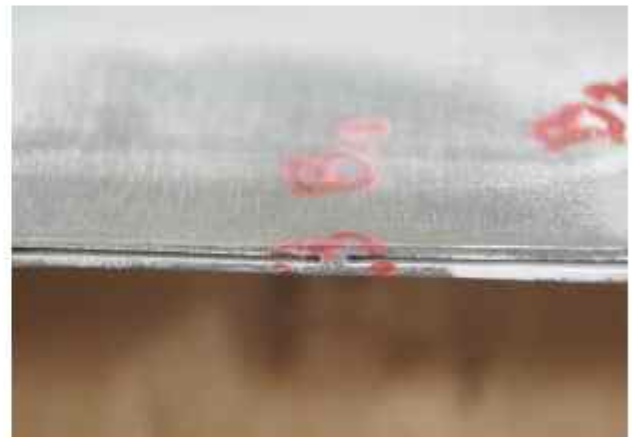
Fig. 4: TURB. BLADE 1 Cracks / Porosity / Roughness - Trailing edge
