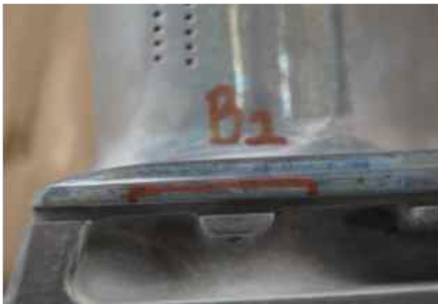
Fig. 3: TURB. BLADE 1 Cracks / Porosity / Roughness - Inner diameter (platform, foot)
