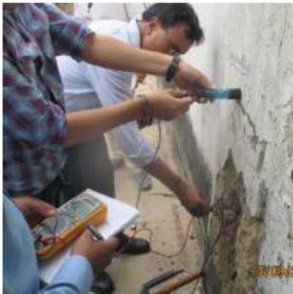
**Fig. 3 Half-Cell Potentiometer test**
