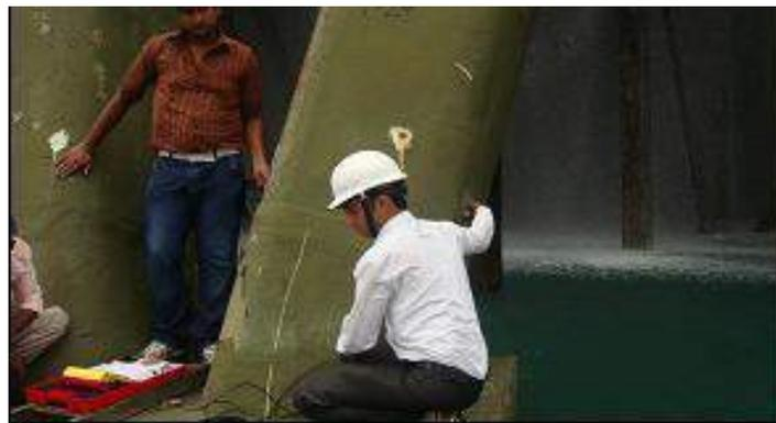
**Fig. 2 Ultrasonic Pulse Velocity test**
