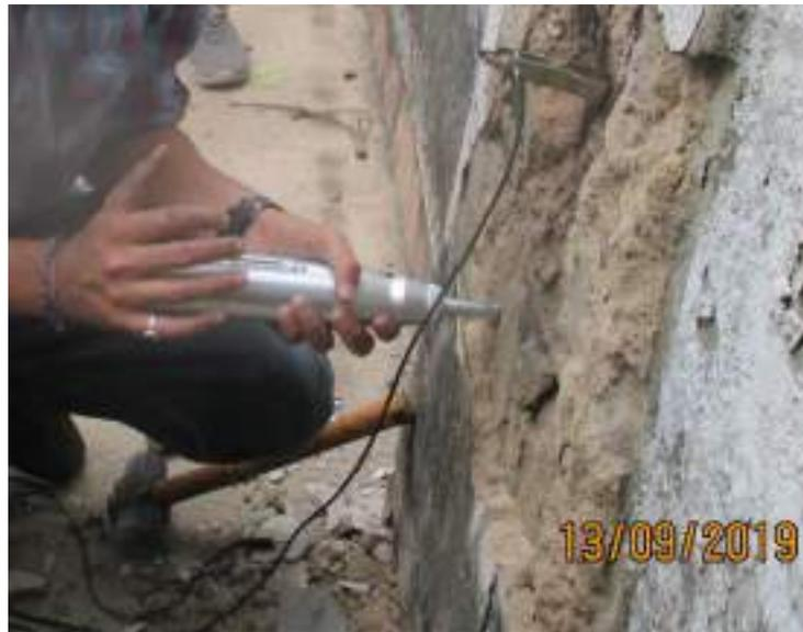
**Fig. 1 Rebound hammer test**
